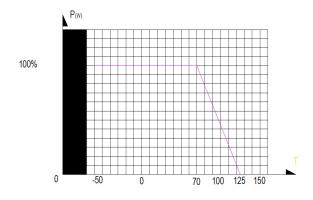
For MELF resistors working at an ambiance temperature of 70°C or above, the power rating shall be derated in accordance with the above curves.
