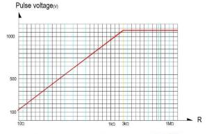
Pulse load rating in accordance with IEC 60115-1,4.27;  $10 \mu s/700 \mu s;$  10 pulses loaded, for permissible resistance change <br/>  $\pm (0.5\% \pm 0.05 \Omega)$
